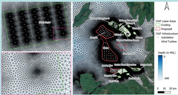
Fig. 4: Eastern Irish Sea TELEMAC model mesh (right), zoomed in on North Hoyle OWF (top left) and an individual monopile (bottom left)
